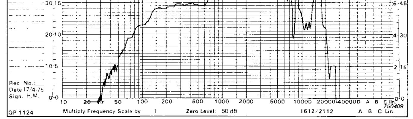
Fig.8. Frequency response of loudspeaker measured with pure sine in anechoic chamber
