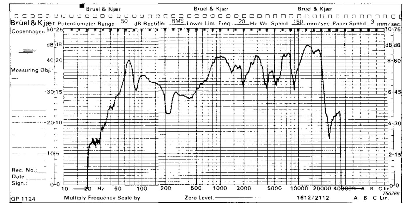
Fig.10. Frequency response of the loudspeaker in Fig.11 measured with Gating System in anechoic room. The difference between these two curves indicates the influence of the Gating System Fig.11. Frequency response of a loudspeaker (not the same as in Figs.8 and 9) using pure sine in anechoic room
