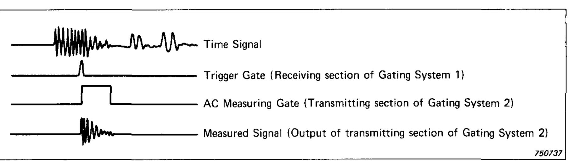
Fig.29. Setting of gates to measure early reflections with the instruments in Fig.28
