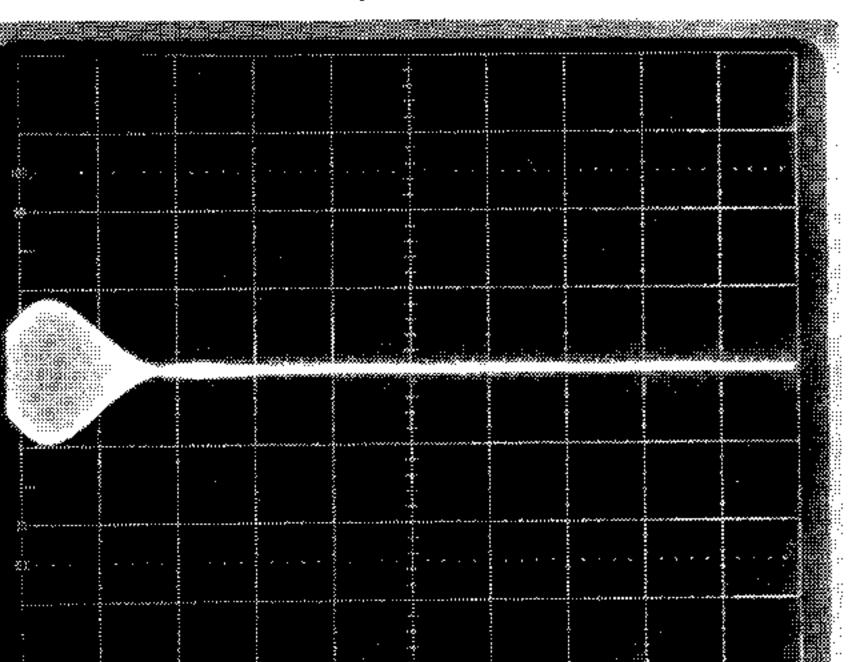
harmonic of the tone burst. Gate is adjusted to measure distortion component
