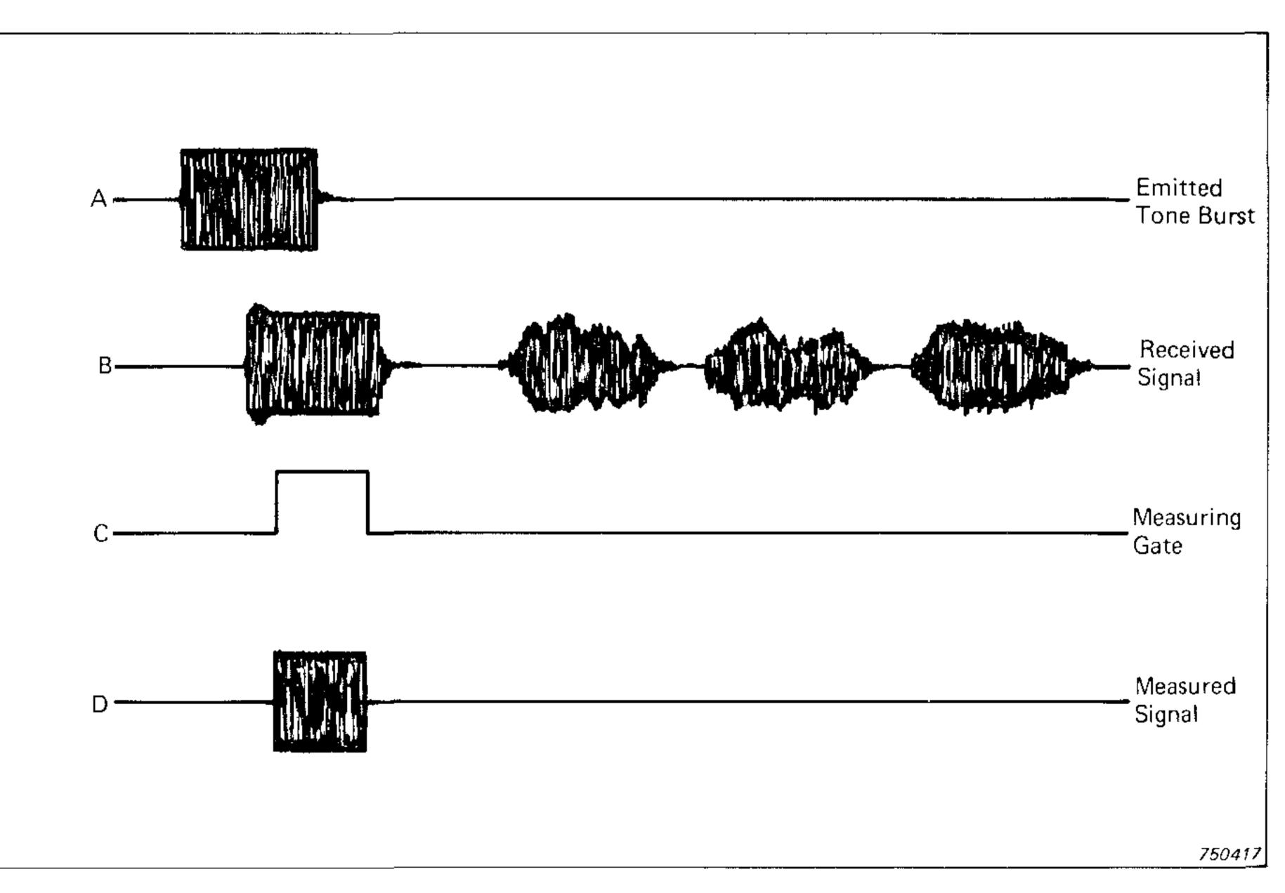
Fig.1. Principle of the Gating System
