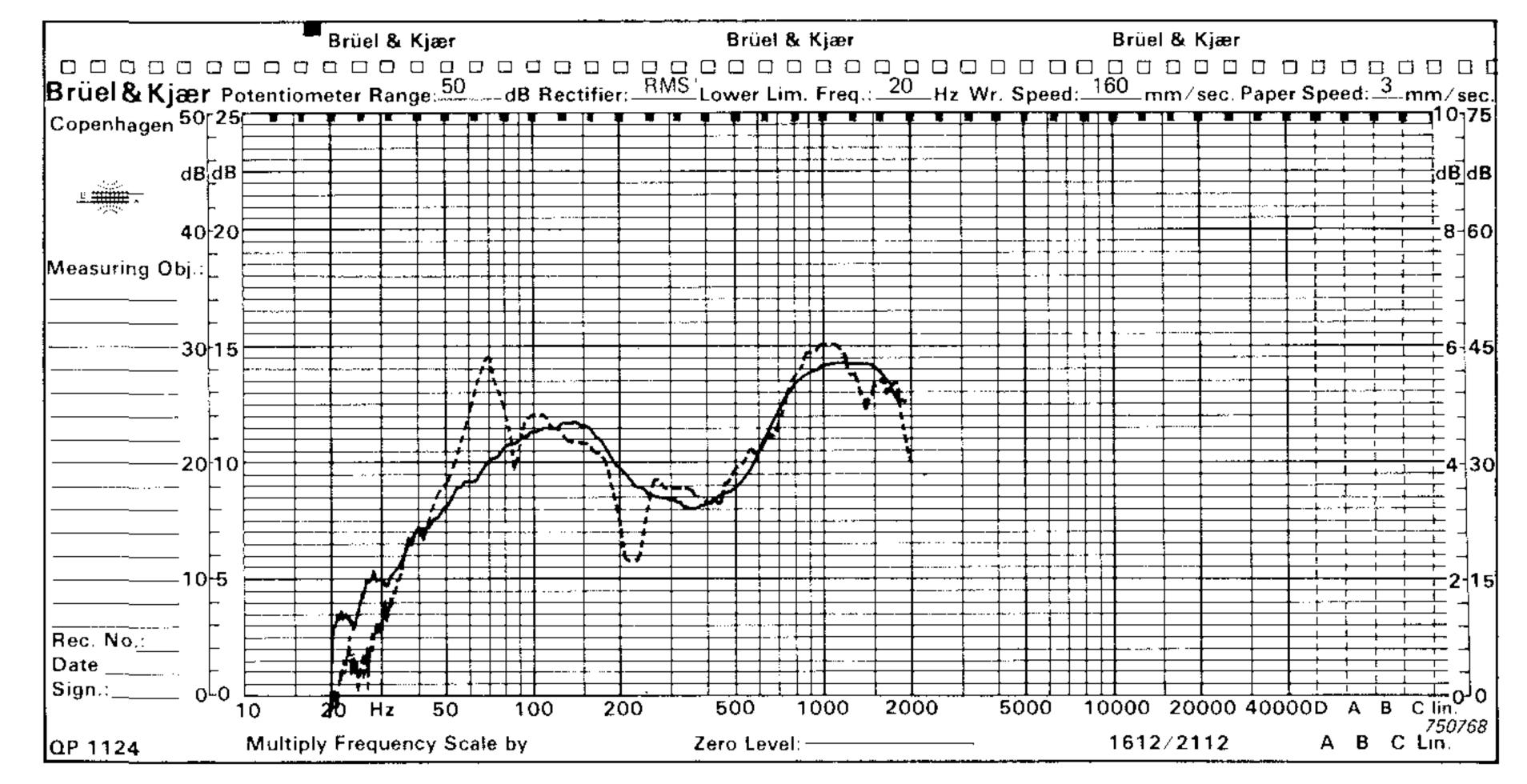
Fig. 18. Illustration of averaging due to too short a tone burst. Dashed line shows free-field
