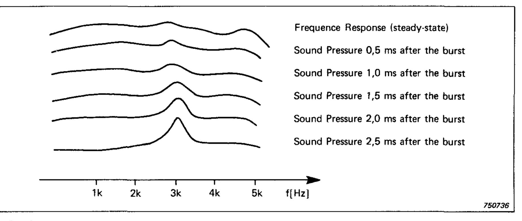
Fig.27. Frequency characteristics of early reflections compared to the steady state response
