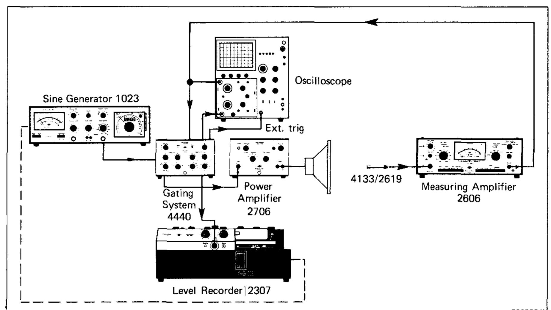
Fig.3. Instrument set-up using the Gating System
